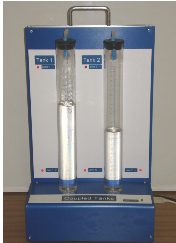
Figure 1. The coupled-tank hydraulic laboratory system uDAQ28/2H
