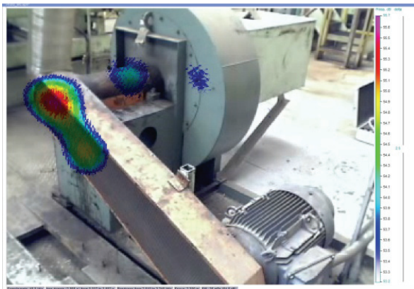
Figure 7. Visualization of the noise emission intensity of fan driving
