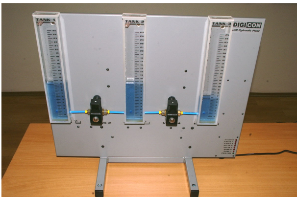
Figure 2. The three-tank hydraulic laboratory system uDAQ28/3H
