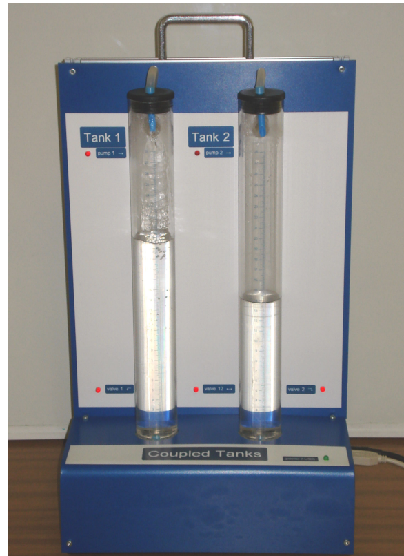
Figure 1. The coupled-tank hydraulic laboratory system uDAQ28/2H
