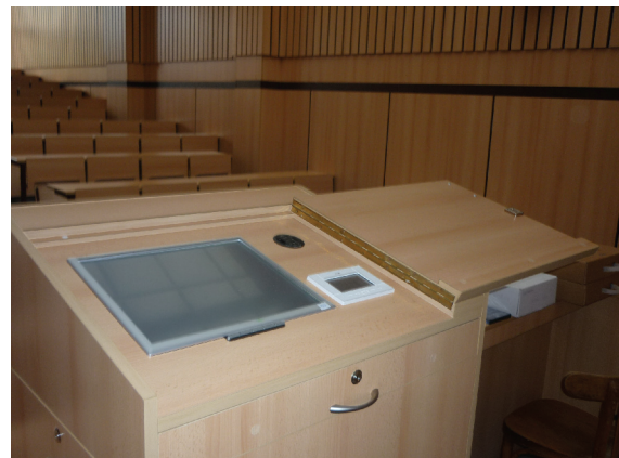
Figure 3. Interactive and control systems of Integrated Multimedia Lecture Desk
